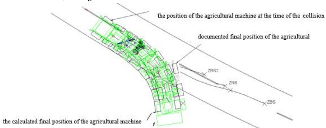
Fig. 4. Representation of the movement of the agricultural machine from the moment of collision to stopping in the final position [11]
